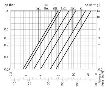
Recommended FLOW RATES to ensure stable operation and an accuracy of  $\pm 2^{\circ}C$
